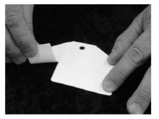
Note: The UHF RFID tag can be read at a distance of 10 meters until the consumer tears it apart, removing the antenna. The RFID tag remains functional but can only be read at a distance of a few centimetres.
