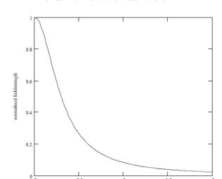
Figure 5. Typical behaviour of the magnetic field strength versus distance (example), for a transmitting antenna with a diameter of 0.8 m.
